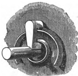
fig. 7. Section to shew the action of wards.
